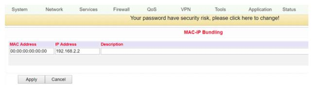
If a firewall blocks all access to the external network, only PCs with MAC-IP bundling will gain access to the external network.
