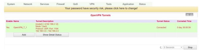
Click *Add* to add a new OpenVPN tunnel. With *Show Detail Status* you can view the status of an already configured OpenVPN tunnel.
