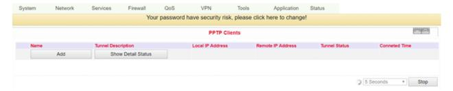
To set up a new PPTP client, click on the Add button. To view details of an existing PPTP client, click the *Show Detail Status* button. When you have clicked the *Add* button, you can make the following configuration settings.
