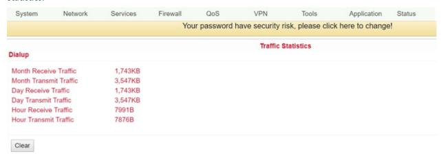
Here you can see the monthly, daily and hourly data that has been received or transmitted. Via the button "Clear" you can reset the entries to 0.
