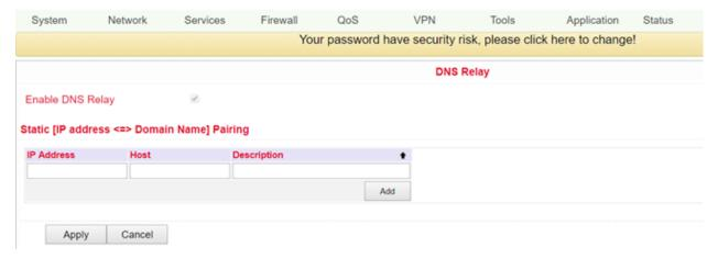
With the *Add* button up to 20 DNS pairs can be created.
