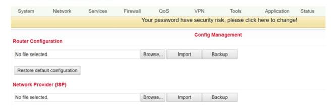
2.) Click *Restore default configuration* to reset the TK500 to its factory settings. After that the router will be rebooted.
