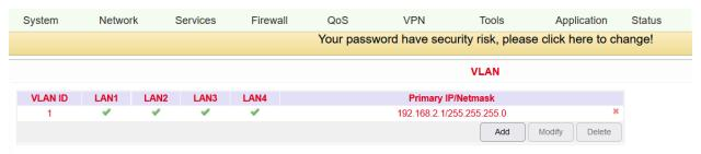
For example, change the IP address to 192.168.1.254 and select the LAN ports to be assigned to this IP address.
