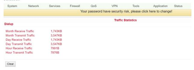
Here you can see the monthly, daily and hourly data that has been received or transmitted. Via the button "Clear" you can reset the entries to 0.
